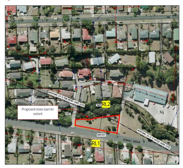
Currently, the predominant noise source is traffic from Dundale Avenue. An ambient noise level of 44dB L<sub>Aeq</sub> was measured on 12 May 2011 at during the day-time.
